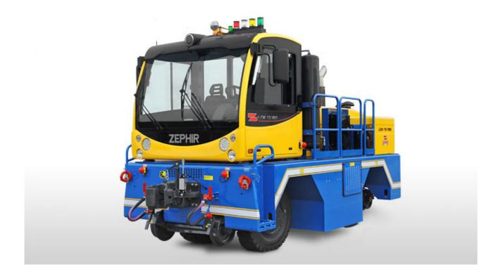
The "LOCOTRACTOR" model LOK is a rail/road Diesel vehicle in accordance to latest CEE rules among which both antipollution and antinoise ones, whose extraordinary versatility cuts down the time taken for rail movements.
