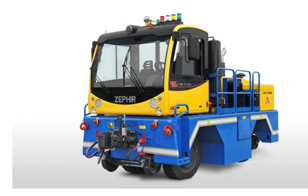
The "LOCOTRACTOR" model LOK is a rail/road Diesel vehicle in accordance to latest CEE rules among which both antipollution and antinoise ones, whose extraordinary versatility cuts down the time taken for rail movements.
