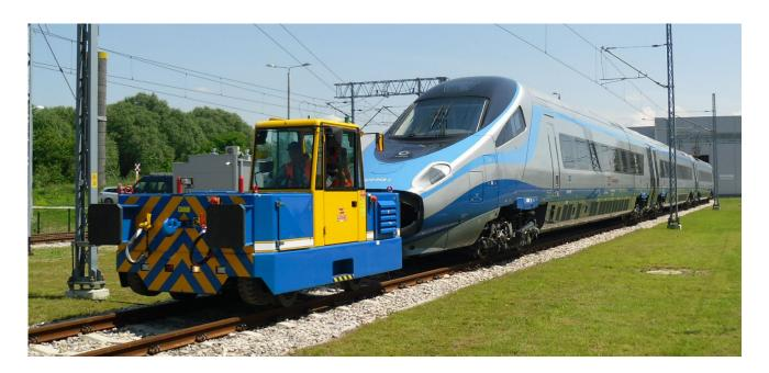
The Zephir CRAB is a road/rail shunter designed to be used in the confined spaces found in rail vehicle maintenance depots. Its compact dimensions and tight turning circle make it easy to manoeuvre within the depot and it is able to enter and leave the tracks in reduced spaces between rail vehicles. The wide range of optional equipment, such as different coupler types, radio remote control and pneumatic braking system air supply, make the CRAB the safest and most effective shunter on the market.
