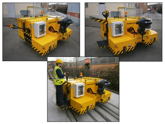
Extra capacity battery: 420Ah, 80V (replaces the standard 350Ah, 80V battery) industrial type, in heavy duty metallic body, centralized refilling system, each element is fitted with visual floater indicating the liquid level. The battery is designed to be easily replaced by the side of the CRAB with the use of a simple forklift truck, or handled through its lifting eyes.
