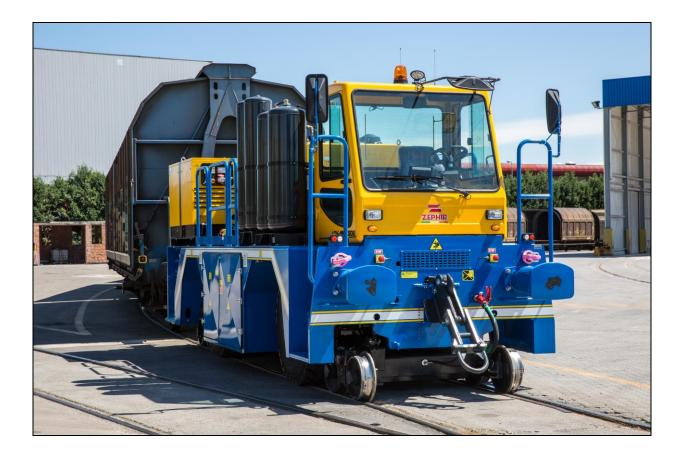
Max draw pull: **160 kN** Max towing/pulling capacity: **3200 t**\* Electric motors: **2x40 kW, 80 V** Battery: **3x1395 Ah, 80 V** Max speed: **6 km/h** (slow gear) – **16 km/h** (fast gear) Nominal weight: **29 t** Dimension (LxWxH): **6500x2500x3200 mm**
