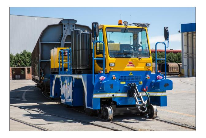
Max draw pull: 200 kN Max towing/pulling capacity: 4000 t\* Electric motors: 2x40 kW, 80 V Battery: 3x1395 Ah, 80 V Max speed: 6 km/h (slow gear) – 16 km/h (fast gear) Nominal weight: 35 t Dimension (LxWxH): 6550x2500x3230 mm
