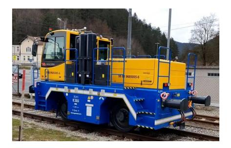
Max draw pull: **70 kN** Max towing/pulling capacity: **1400 t**<sup>\*</sup> Electric motors: **2x32 kW, 80 V** Battery: **2x930 Ah, 80 V** Max speed: **7 km/h** (slow gear) – **15 km/h** (fast gear) Nominal weight: **24 t** Dimension (LxWxH): **4800x2500x3400 mm**
